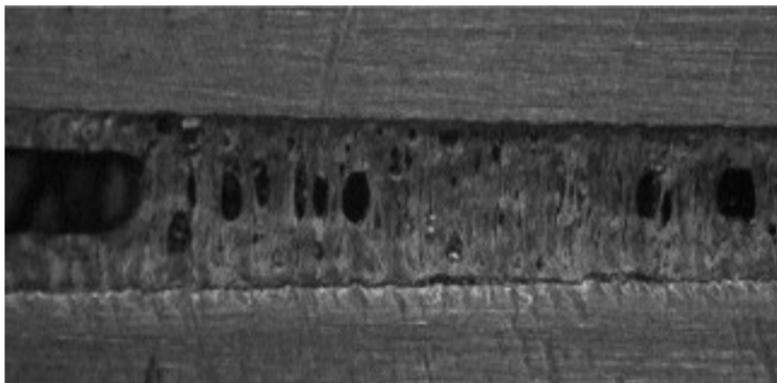
Failure process of a porous adhesive joint in opening mode fracture [Zhu-Liechti-Ravi-Chandar '09]
