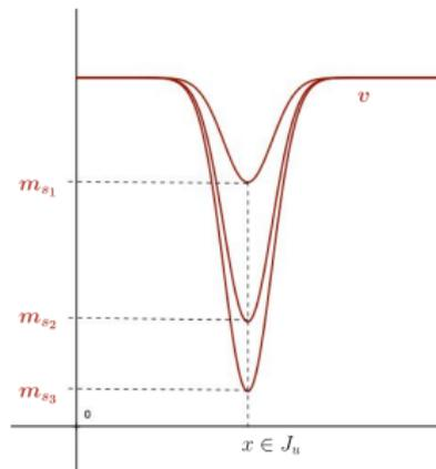
**Bar in traction.** Distributions of displacement  $u$  and of damage  $v$  along the bar for different values of the imposed displacement, in the case  $f_\delta(v) := \min\{1, \delta v^2 / (1 - v)^2\}$ .
