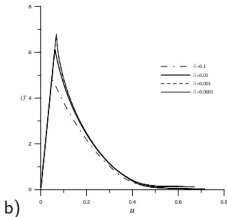
**Bar in traction.** Left: graph of the cohesive energy density  $g_{\text{scal}}([u])$ . Right: stress  $\sigma$  as a function of the imposed boundary displacement, for different values of the small parameter  $\delta$ .
