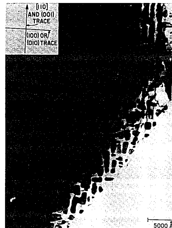
Figure 72. Cuboidal precipitates in the Cu-22.0 Au alloy (187). (Courtesy of M. J. Marcinkovski and L. Zwell.)
