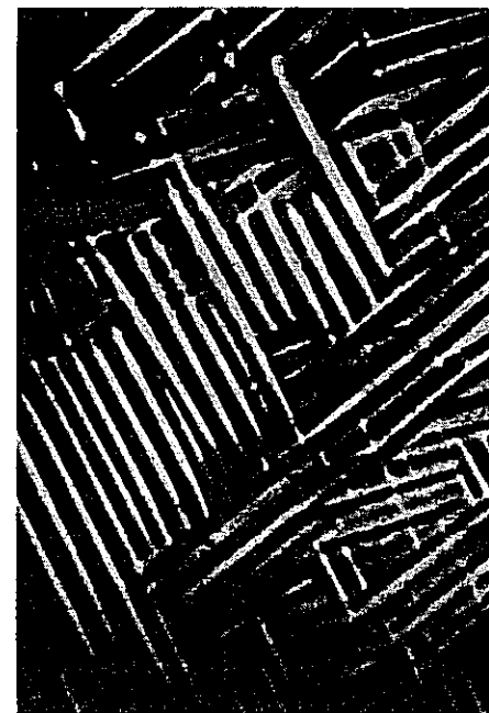
Figure 87. Electron micrograph of complexes of one-dimensional modulated structures in a Fe-Si alloy (217). \times 35,000 . (Courtesy of H. Warlimont.)
